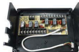
RE392 6 ZONE RELAY BOARD IN ENCLOSURE TO SUIT RE390
